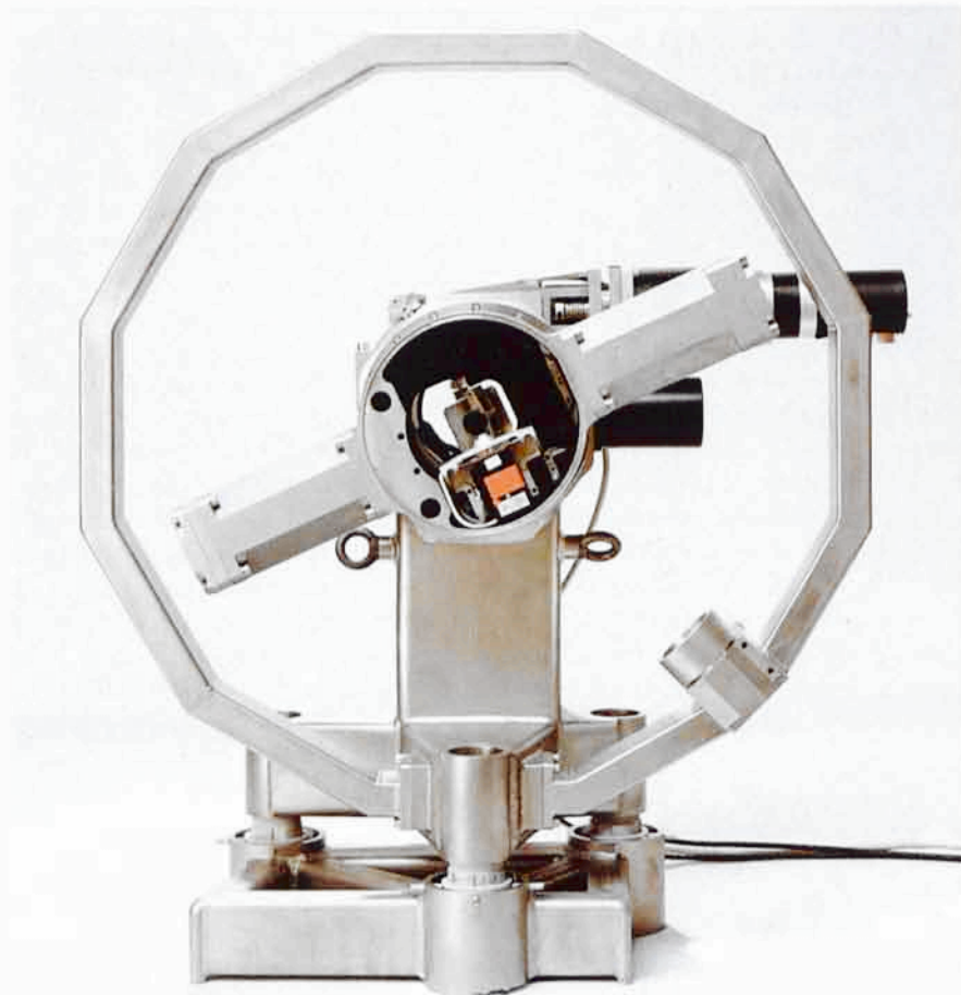
IRSPEC de-rotator at the NTT. This rotating three-mirror device is mounted between the spectrometer and the Nasmyth adapter where it is used to set the desired slit position angle, counter the field rotation at the Nasmyth focus and also acts as a focal reducer and a focal plane sky chopper.
