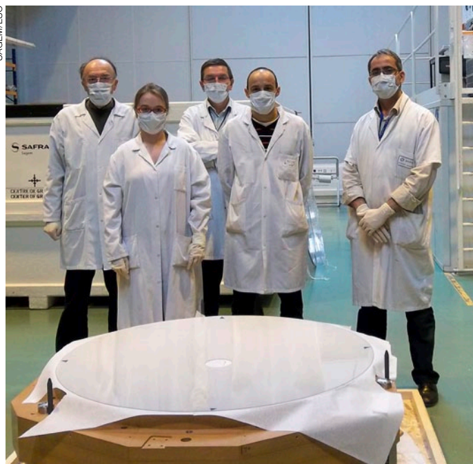
Engineers at SAGEM (France) stand behind a remarkable thin-shell mirror that they have created for the Very Large Telescope Adaptive Optics Facility. The front convex face is the optical surface and the concave face will be equipped with 1170 small magnets glued on the surface allowing controlled deformation via forces applied by voice coil actuators. The shell is 1120 millimetres in diameter and 1.998 millimetres thick.
