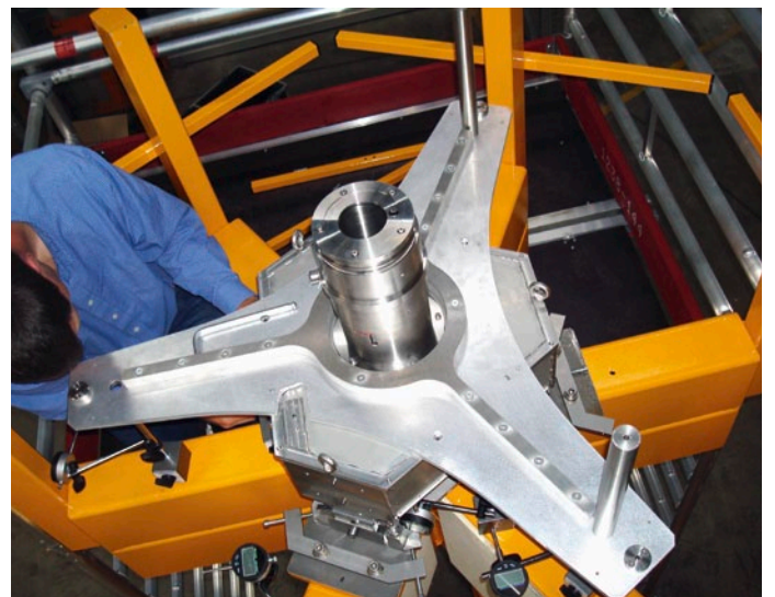
E-ELT primary mirror test stand equipped with dial test indicators in preparation for laser tracker tests.
