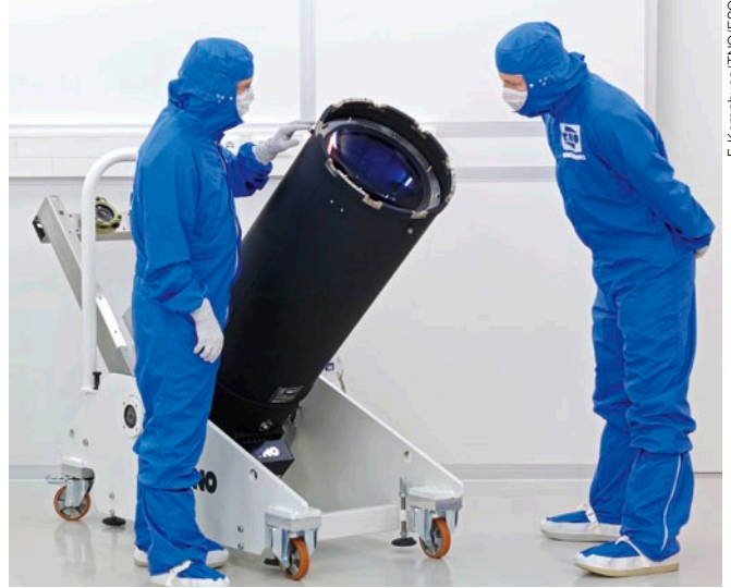
The first optical tube assembly unit completely assembled in TNO's cleanroom in the Netherlands.
