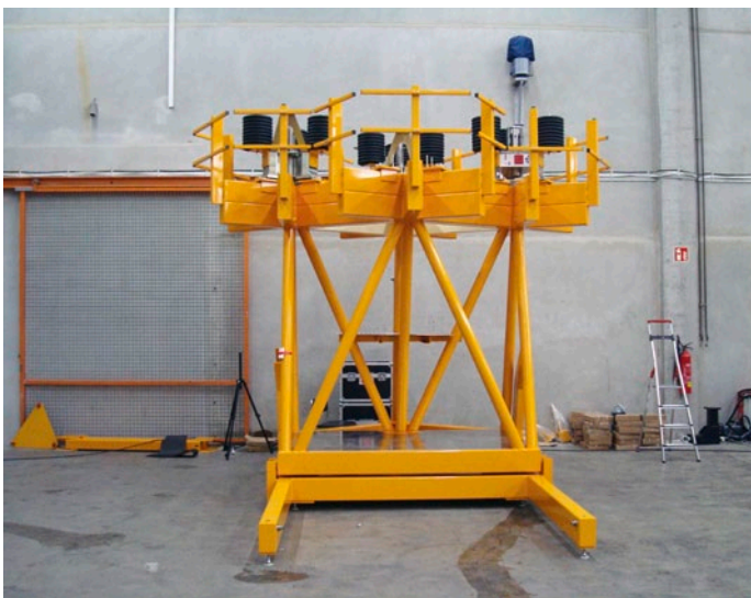
E-ELT primary mirror test stand fully loaded with four fixed frames and dummy masses.
