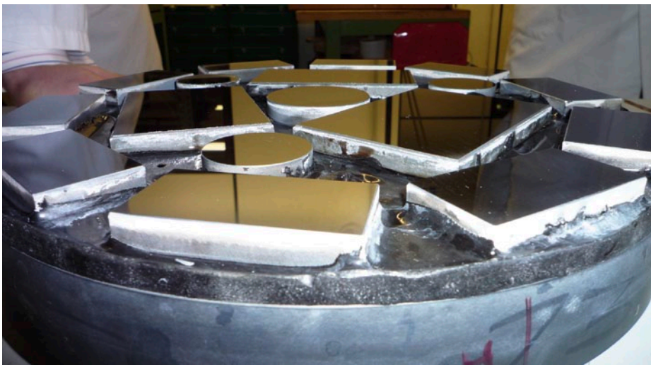
Silicon carbide mirrors during the polishing process.
