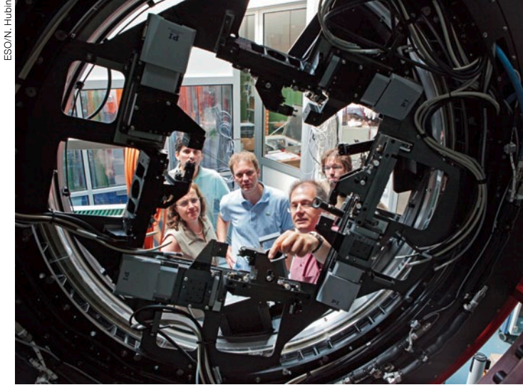
GRAAL main assembly in the ESO integration hall with optics installed.
