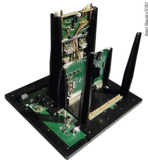
Digitiser test equipment serves as a trouble-shooting tool for the ALMA digitiser.
