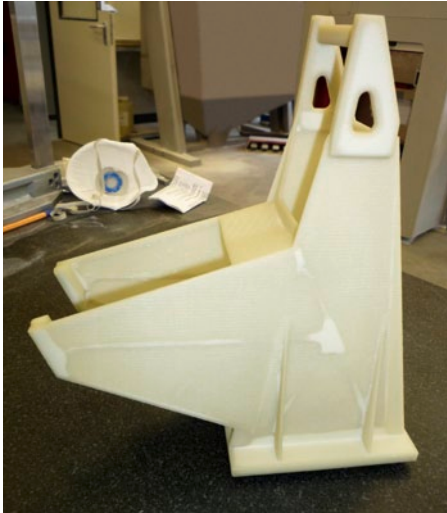
3D "print" of a wax-impregnated mould.
