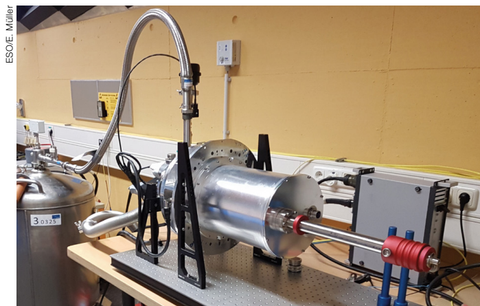
CCD qualification setup with iron-55 source.
