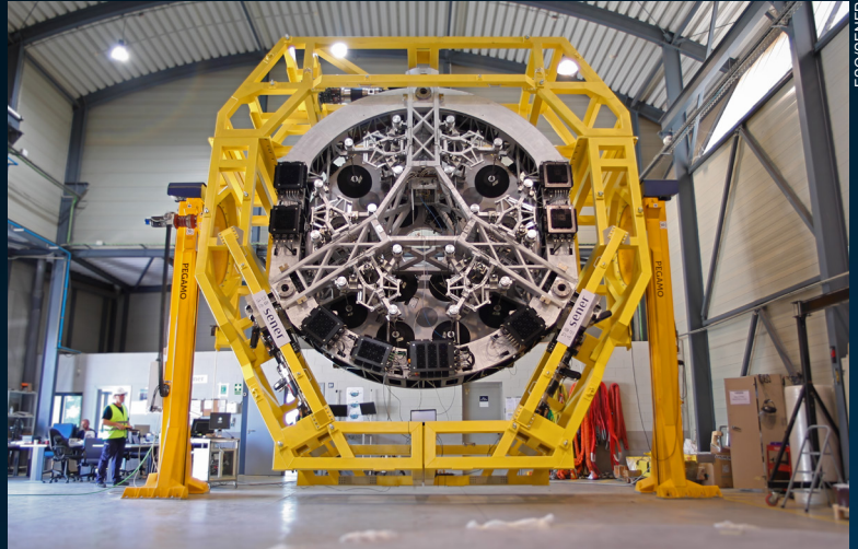
Testing of the ELT M2 mirror cell.
