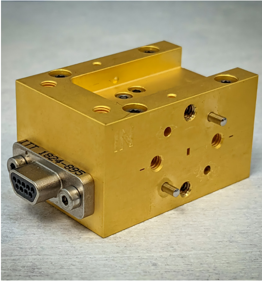
Cryogenic low-noise RF amplifier for the frequency range 125–211 GHz.
