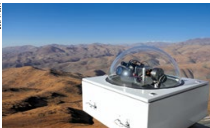
The HELIOS solar telescope attached to the catwalk of the ESO 3.6-metre telescope at La Silla.
