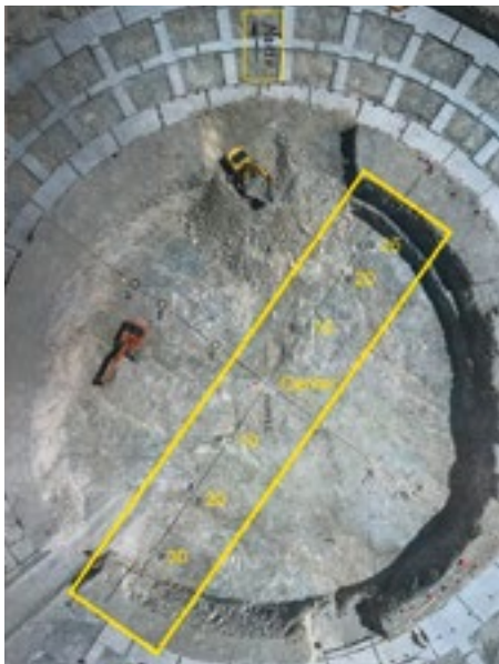
Measuring soil resistivity on the Armazones platform.
