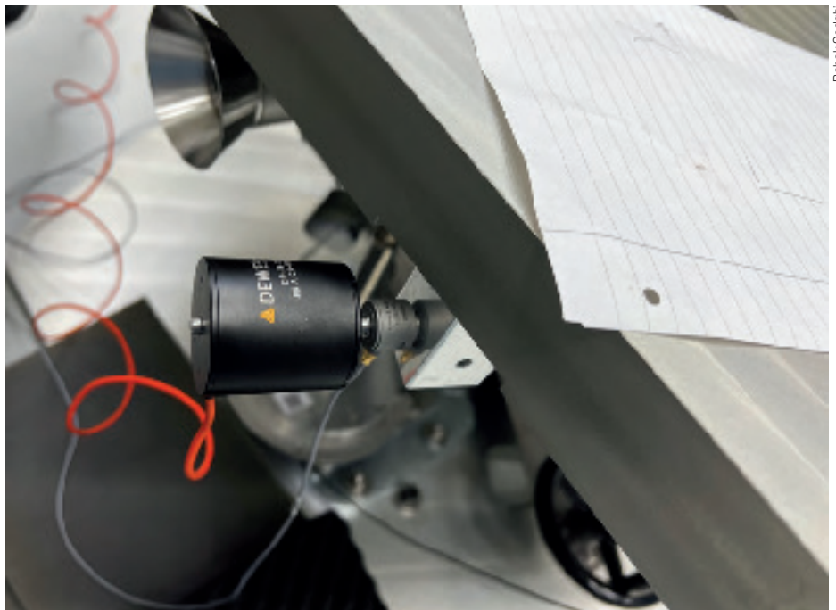
Inertial exciter together with a force sensor connected to an ELT M1 segment, for performing modal tests.
