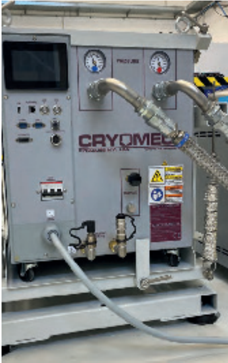
Large Integration Hall vibration testing facility: Measuring exported forces of a cryo-compressor (variable speed) isolated by a double stage anti-vibration
