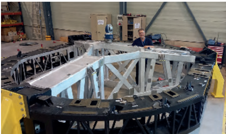
The M2 and M3 cells developed by SENER completed their final design phase and underwent manufacturing during 2021. Here, the M2 cell structure is seen during its integration.
