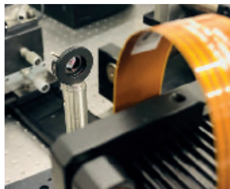
R&D in optical surface testing, using a spatial light modulator as a programmable computer-generated hologram.
