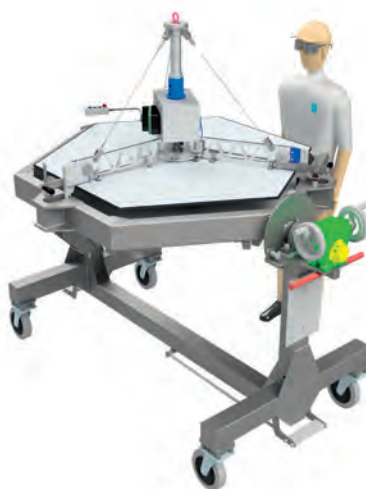
CAD design of M1 segment gripper and transportation cart for handling activities in the ETF.
