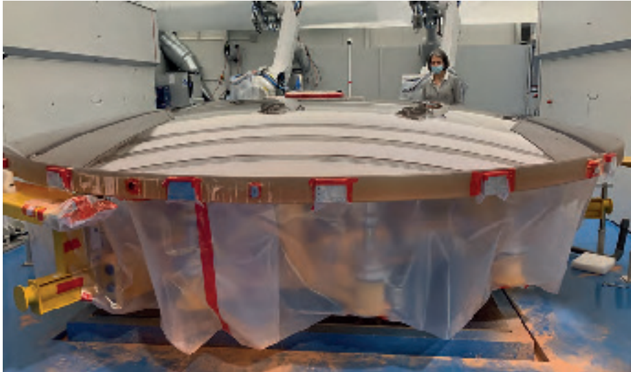
The 4.2-metre-diameter ELT secondary mirror (M2) went through its pre-polishing phase at Safran Reosc in 2021, reaching a surface accuracy of about 2 \mu\text{m} rms.
