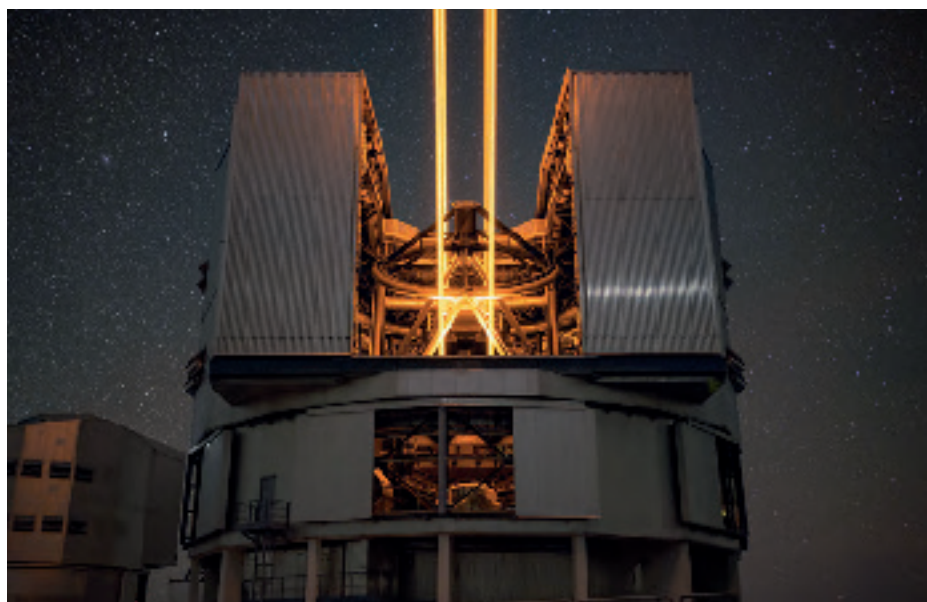
The four beams of the Adaptive Optics Facility laser guide stars emerge from the VLT's Unit Telescope 4 at Paranal.
