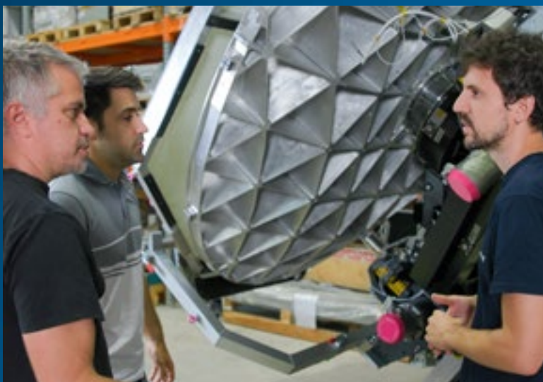
View of the rear side of the ELT M5 mirror blank.
