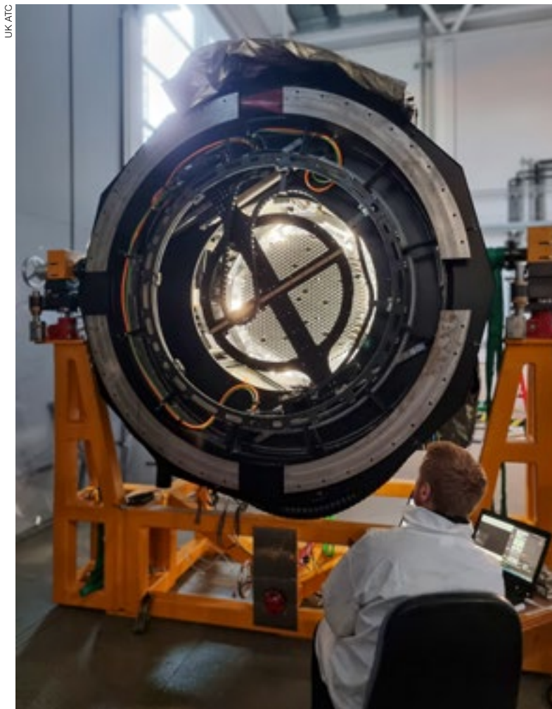
The rotating front end of MOONS, with the metrology lights illuminated.
