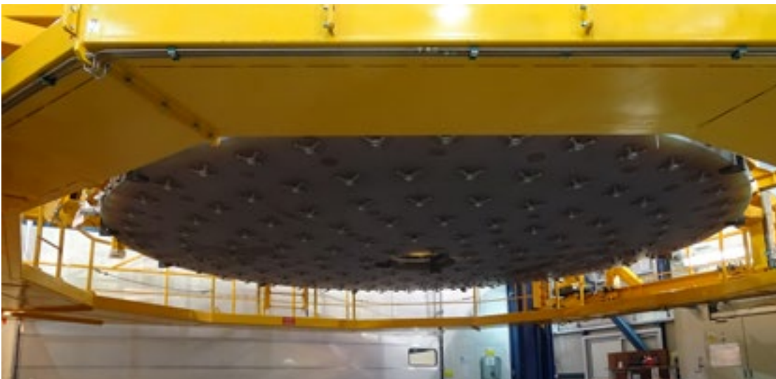
The VLT M1 Mirror Handling Tool is used to move the VLT's 23-tonne, 8.2-metre-diameter primary mirrors when they need to be recoated.
