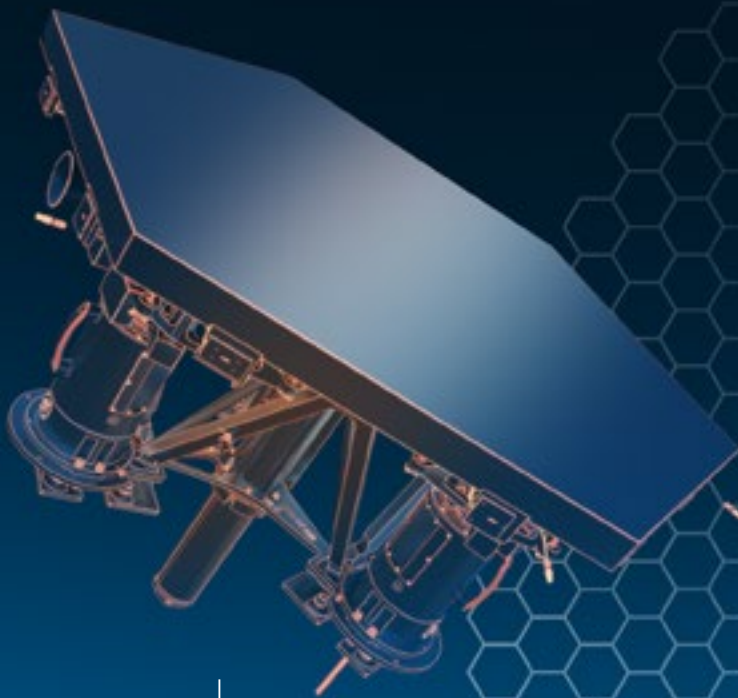
Artist's impression of one of the 798 segments of the ELT's primary mirror.
