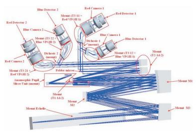
Figure 4.5. The optomechanical concept of the CODEX spectrograph.
