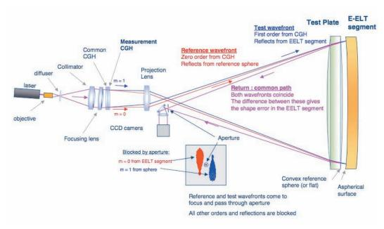
Figure 3.90. Sagem's (Arizona mirror lab) proposed test setup for final production.
