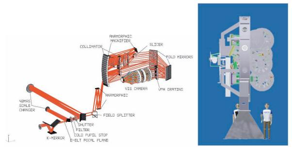
Figure 4.8. The optical path of a single channel from the K-mirror that de-rotates the field to the detector. This is for one of the two visible cameras. Light from the telescope passes through the scale changer in the fore-optics, then is subdivided at the field splitter. The beam is collimated before entering the slicer and finally focused onto the spectrometer  $4k \times 4k$  array.
