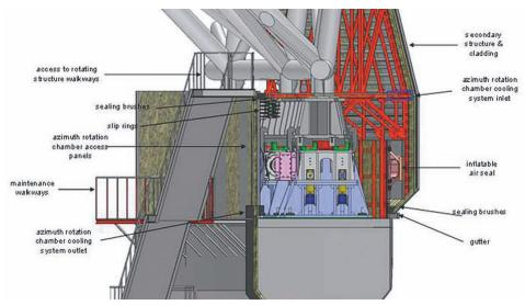
Figure 3.27. The azimuth rotation chamber.
