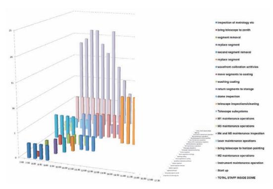
Figure 5.4. Plan for the execution of the preventive maintenance tasks inside the E-ELT dome.
