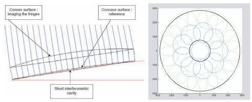
Figure 3.124. Mirror testing using test matrices and stitching.
