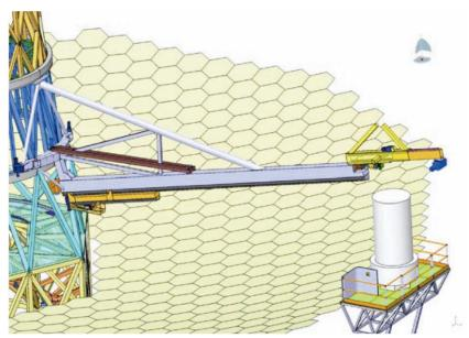
Figure 3.60. The retractable platform and segment lowering operation.
