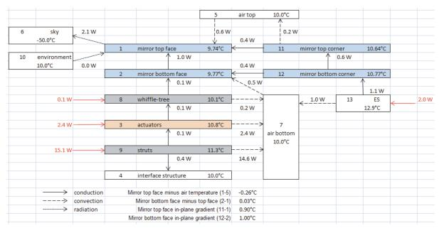
Figure 3.112. Simplified lumped parameter network showing the main of heat fluxes.
