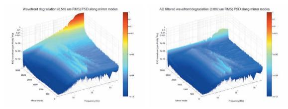
Figure 3.107. Frequency distribution of WFE (before and after adaptive correction).
