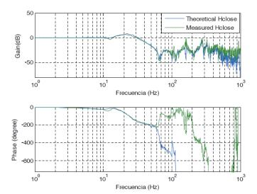
Figure 3.99. Measured closed-loop transfer function of the actuator with an equivalent segment mass attached.
