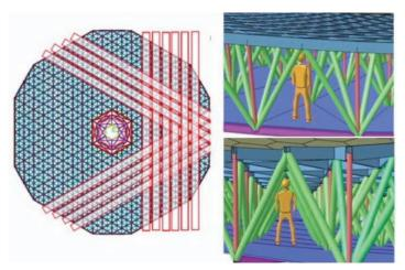
Figure 3.48. The telescope mirror cell structure.
