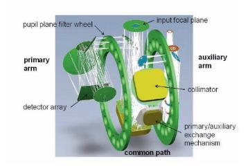
Figure 4.10. The two arms of the MICADO instrument — the primary arm with the 53 arcseconds × 53 arcseconds camera and 16-detector focal plane; the auxiliary arm with the additional scientific modes including spectroscopy, higher resolution imaging at 1.5 mas per pixel and options include high time-resolution imaging, polarimetry. A simple fold mirror is used to select between them.
