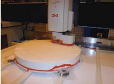
Figure 3.91. Apherising and pre-polishing at Sagem.
