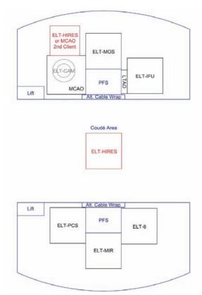
Figure 4.1. A possible arrangement for the instruments on the Nasmyth platforms and coudé area.
