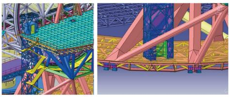
Figure 3.58. Lift for human and tool access to the Nasmyth platforms.
