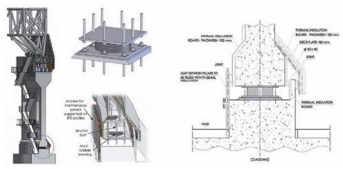
Figure 3.38. Location of the dome seismic isolators.
