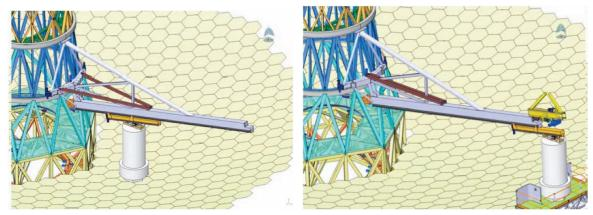
Figure 3.59. The jib crane mounted on the central tower.
