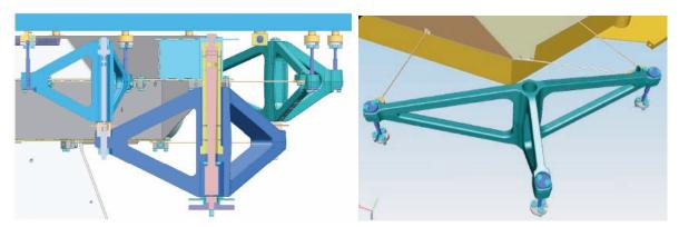
Figure 3.70. Left: Whiffletree struts. Right: Axial and lateral.
