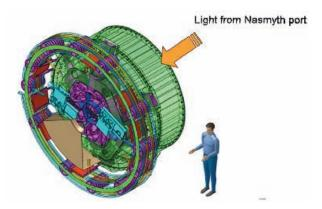
Figure 4.3. The ATLAS post-focal laser tomography AO module.
