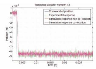
Figure 3.158. Step response of a single actuator — simulation and measurement.
