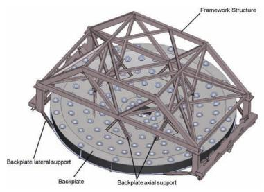
Figure 3.126. Steel framework structure and CFRP backplate.
