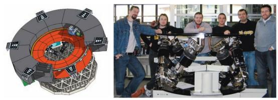
Figure 3.152. M4 mounting structure and positioning system for the Dark Energy CAMera.
