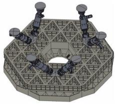
Figure 3.148. The reference body with hexapod legs.
