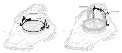
Figure 3.36. Selected images from the erection sequence of the dome.
