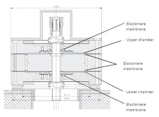
Figure 3.128. Pneumatic actuator. The pressure in the two chambers provides stiffness; the differential pressure between the two chambers allows force adjustment.
