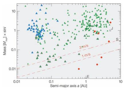
Figure 2.2. Mass plotted against semi-major axis of known exoplanets. The stars currently detected through the radial velocity technique (green triangles) are limited by the accuracy of ~ 1 ms<sup>-1</sup>, while the E-ELT will push the limit to < 10 cms<sup>-1</sup>, allowing Earth twins (marked as "E") to be detected. Credit: Bouchy et al. (2009).
