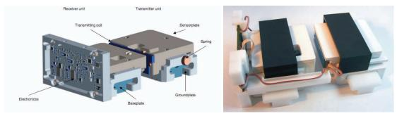
Figure 3.100. Left: Edge sensor components. Right: Prototype edge sensor devices.
