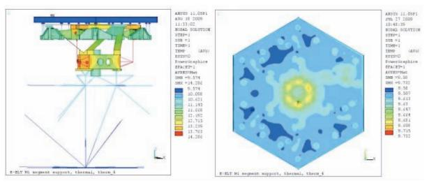
Figure 3.113. Thermal analysis for the segment.
