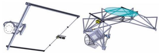
Figure 3.187. Adaptive optics calibration unit trolley and structure supporting the projector.
