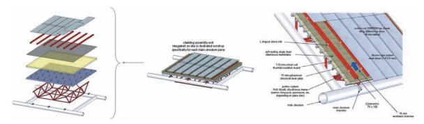
Figure 3.30. Details of the cladding structure.
