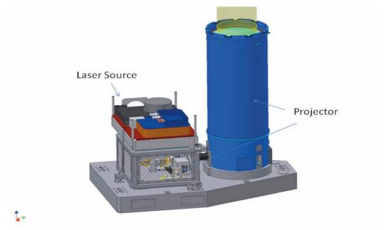
Figure 3.184. Laser guide star unit of the Four Laser Guide Star Facility (main optomechanics).
