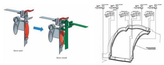
Figure 3.24. Door seals and water-labyrinth scheme.
