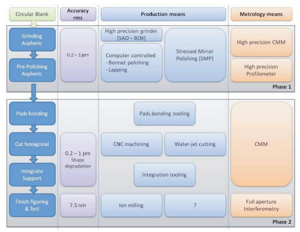
Figure 3.81. M1 segment assemblies — figuring process.
