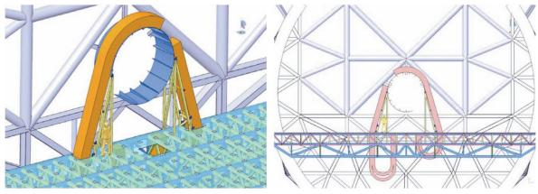
Figure 3.54. Altitude cable wrap.
