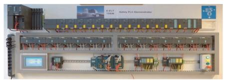
Figure 3.193. The scale-one demonstrator of the interlock and safety system.
