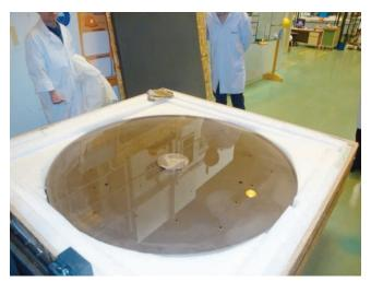
Figure 3.115. ULE polished segment before cutting at Sagem.
