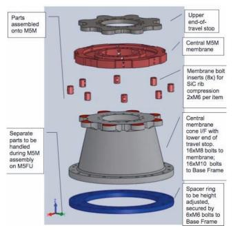
Figure 3.164. Components of the central restraint.
