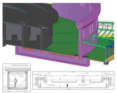
Figure 3.18. Gallery for telescope supplies.
