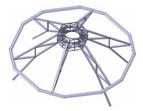
Figure 3.50. The spider and secondary mirror crown.
