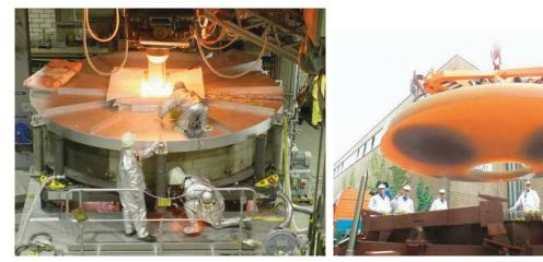
Figure 3.121. Schott 4-metre blank. Left: Casting. Right: Finished product (Courtesy Schott).
