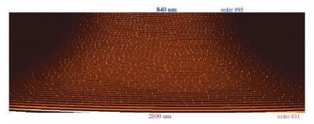
Figure 4.17. The SIMPLE echellogram on  $3 \times 4k \times 4k$  arrays.
