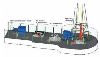
Figure 3.122. Possible M2 polishing workshop — modifications of VLT Primary Mirror workshop (courtesy Sagem).
