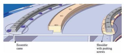
Figure 3.174. The concentric rails for the adapter and the rack for the drive units.
