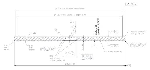
Figure 3.83. Segment blank dimensions.
