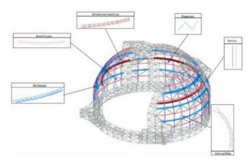
Figure 3.20. The dome secondary structure.
