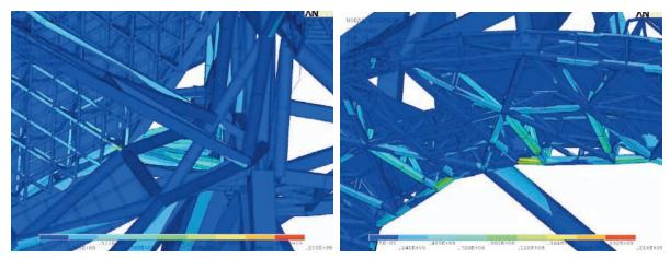
Figure 3.63. Maximum stress distribution in the M1 cell (left) and azimuth floor (right) in Pa.
