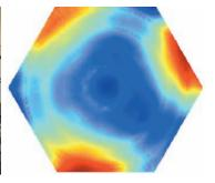
Figure 3.86. Left & centre: The stress mirror fixture from Tinsley. Right: Segment residuals from the Tinsley process (3 µm peak) (hexagonal extract from oversized polished surface).
