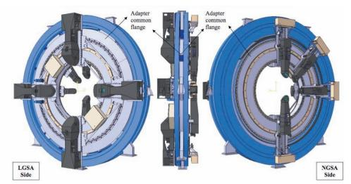
Figure 3.170. Laser and natural guide probe adapters.
