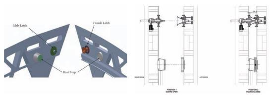
Figure 3.23. Door latching mechanism.
