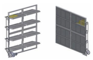
Figure 3.31. Louver design in open and closed configurations.
