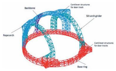
Figure 3.19. The dome primary structure.
