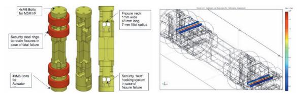
Figure 3.165. Axial flexures connecting the mirror interface to the actuators and the stress calculation for flexures.
