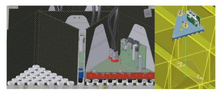
Figure 3.150. A brick interfacing with the borosilicate inserts and being inserted into the structure.
