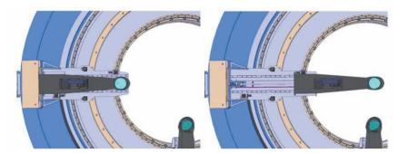
Figure 3.173. The guide probe retracted and extended.
