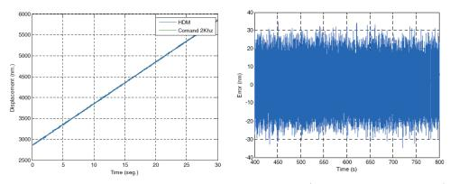
Figure 3.98. Lab measurements of the actuator tracking a ramp of 100 nms<sup>-1</sup> over several minutes. Left: Snapshot of the absolute measurement using the internal Heidenhain encoder. Right. The residual of 7.31 nm rms, including the major contributions from the lab environment.
