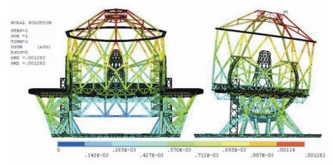
Figure 3.53. Displacement due to a temperature gradient of 0.05°Cm<sup>-1</sup> along y.
