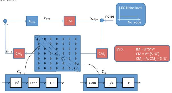
Figure 3.106. Closed loop control, different controllers for different spatial frequencies.
