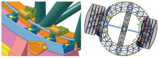
Figure 3.47. The altitude support assembly and identification.
