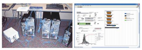
Figure 3.195. Off-the-shelf computers demonstrating the telescope RTC and timing tests on prototype RTC.
