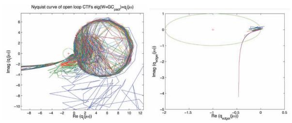
Figure 3.108. Stability analysis for position actuator and edge sensor loops (Nyquist curves).
