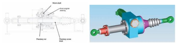
Figure 3.130. Position actuator components and CAD view.
