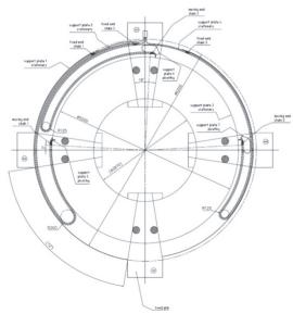
Figure 3.175. The natural guide star cable wrap system.
