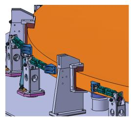
Figure 3.141. Earthquake safety clamps on the tertiary mirror.
