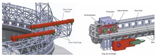
Figure 3.22. The door tracks and bogie.
