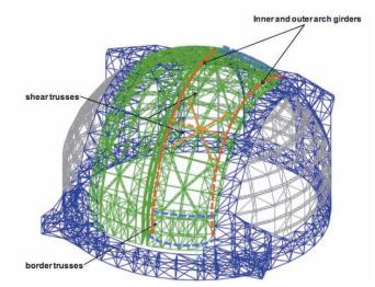
Figure 3.21. The structure of the doors.
