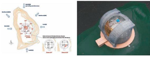
Figure 3.39. Test scenarios and the dome model for the wind tunnel study.
