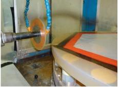
Figure 3.92. Medium-sized tool smoothing and cutting before ion-beam touching up.
