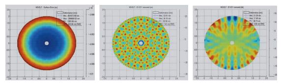
Figure 3.143. Gravity deformation of the tertiary mirror and deformation of the tertiary mirror after removal of the first 11 elastic mode terms and lateral support residuals.
