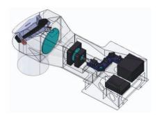
Figure 3.177. The laser guide probe.
