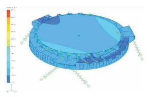
Figure 3.140. First mode of the system at 8 Hz.
