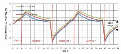
Figure 3.114. Transient thermal analysis for individual segments in a no-wind analysis.
