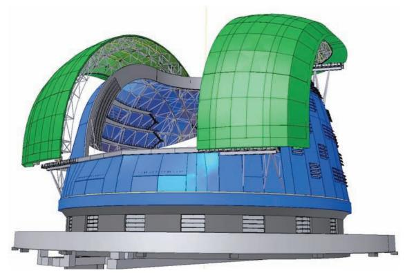
Figure 3.41. EIE/Cimolai alternate dome FEED design.
