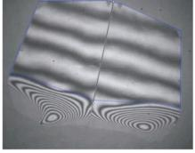
Figure 3.157. Prototype and demonstration of the phasing of thin sheets. The piston sensing unit in front of the demonstration prototype (left) and fringes across two segments at the demonstration prototype (right). The lower regions are deformed due to the supporting structure and are not part of the useful area.
