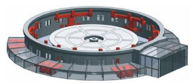
Figure 3.32. The distribution of the air handling units and ducting.
