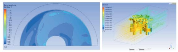
Figure 3.110. Left: Temperature of front face of primary mirror under 2 ms<sup>-1</sup> wind loading. Right: Simplified segment support used for airflow calculations.
