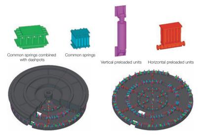
Figure 3.17. Seismic isolation proposal for the telescope foundations.
