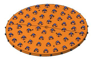
Figure 3.134. Back-side interface tripods on the mirror.
