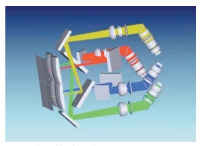
Figure 4.13. The optical layout of OPTIMOS–DIORAMAS in spectroscopic mode showing the four optical paths that make up the instrument — two optimised for the  $0.6-1.4 \, \mu m$  range and two for the  $0.37-1.0 \, \mu m$  range.
