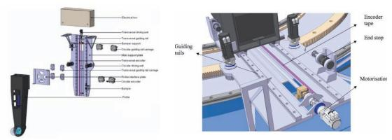
Figure 3.172. The components of the translation stage.
