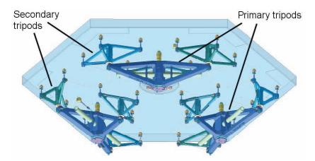
Figure 3.69. The whiffletree structure.
