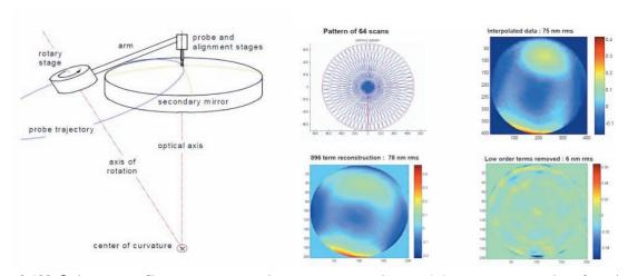
Figure 3.123. Swing-arm profilometer concept and measurement results on a 1.4-metre convex asphere from the University of Arizona.
