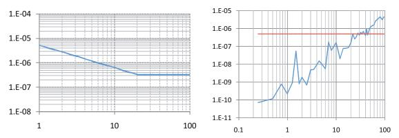
Figure 3.34. Track smoothness in m vs. Hz (rotational frequency) and acceleration per square root of frequency vs. frequency (g/\JHz vs. Hz).
