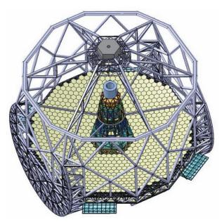
Figure 3.46. The altitude structure of the telescope.
