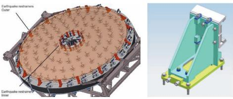
Figure 3.132. Safety restraint for the secondary mirror.
