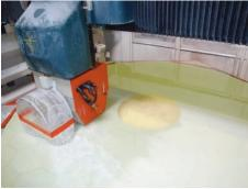
Figure 3.155. The 2.7-metre 2 mm thin shell on the blocking body and in the thinning process.
