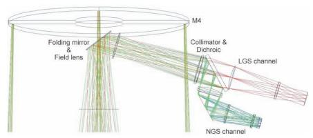
Figure 3.186. Optical design of the beam projection unit.
