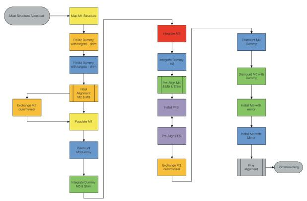
Figure 3.197. Optical pre-alignment flow diagram.
