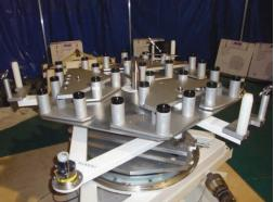
Figure 3.89. Left: 3D-Coordinate Measuring Machine. The baseline optical profilometer to be used during aspherisation. Right: The metrology whiffletree.
