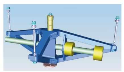
Figure 3.71. Segment shape counterweights.
