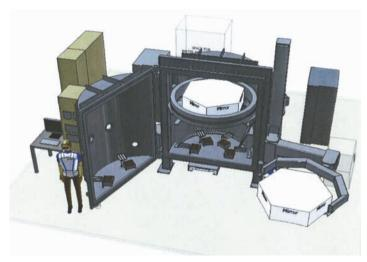
Figure 3.8. Segment coating unit.
