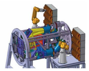
Figure 4.12. A view of the OPTIMOS–DIORAMAS system with the cabinets for the filters and gratings and robotic exchange mechanisms (to the right). At the left of the figure, the mask exchange mechanism can be seen. The cylindrical structure is the rotating part of the instrument.
