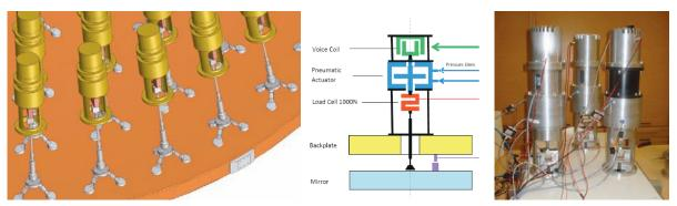
Figure 3.129. Shape actuators.
