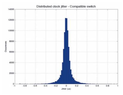
Figure 3.192. Measured jitter on the timing signals across IEEE1588.
