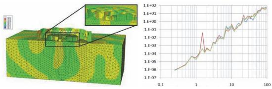
Figure 3.33. Model for the calculation of the transfer function from the dome bogies to the telescope foundations and transfer function in units of ms<sup>-2</sup>/m vs. Hz.
