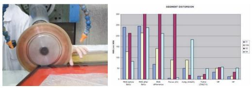
Figure 3.87. Segment cutting and measured segment distortion after cutting (s1/blue Zerodur, s3b/yellowAstrosital, s2/red & s4/cyan ULE).
