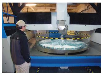
Figure 3.85. Large-scale Zeeko polishing machine at Optic Glyndwr.
