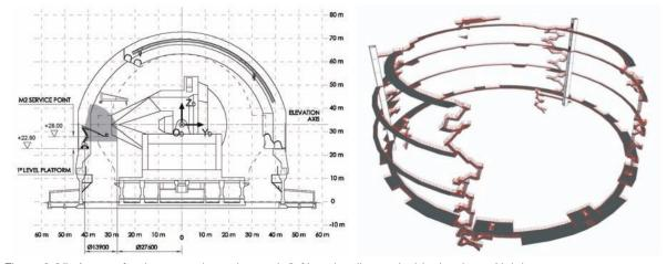
Figure 3.35. Access for the secondary mirror unit (left) and walkways inside the dome (right).
