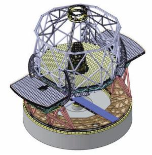
Figure 3.65. The complete main structure erected including all 798 dummy segments.
