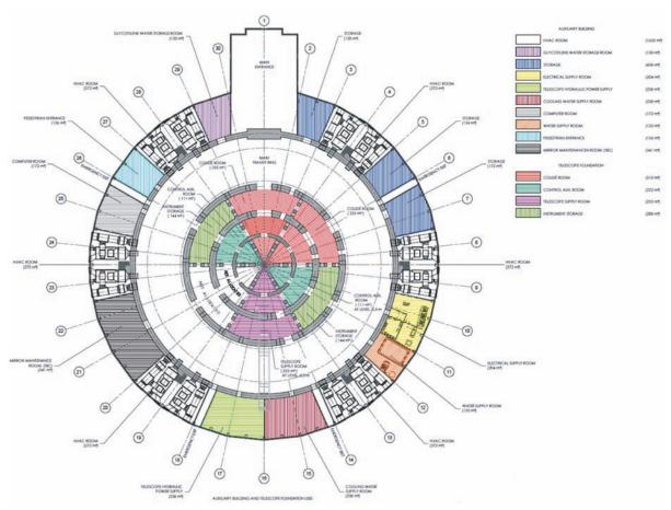
Figure 3.11. Minimalist site footprint including the coating chambers and instrument handling in the dome.
