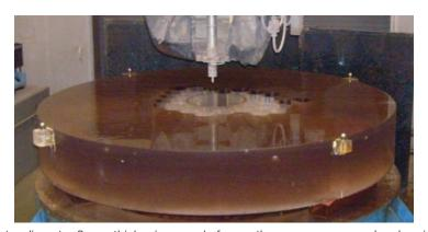
Figure 3.160. A 2-metre diameter 3 mm thick mirror made for another programme, under abrasive water-jet cutting. The final mirror had significantly better performance than our specifications.
