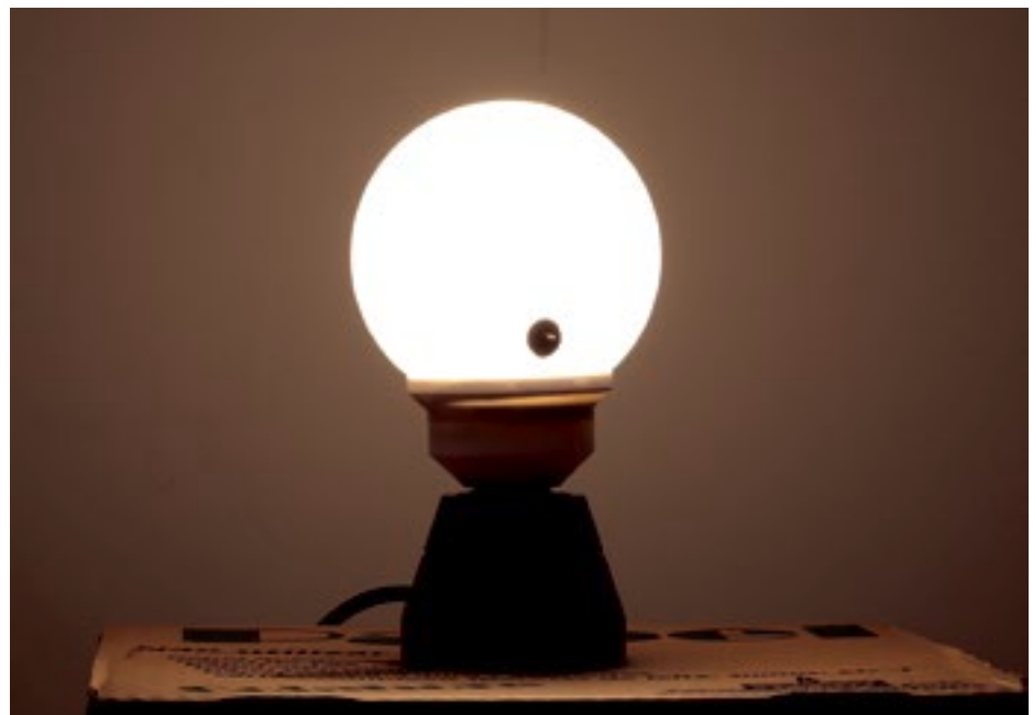
Figure 1. One of the pictures taken to simulate the transit method for detection of exoplanets. A small ball held by a thread is photographed at multiple positions while crossing in front of the bulb. Credit: Pedro Mondim and Pedro Pedrosa
