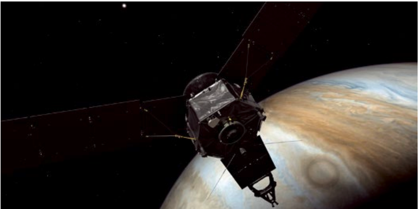
Figure 1. This artist's illustration depicts NASA's Juno spacecraft at Jupiter, with its solar arrays and main antenna pointed towards the distant Sun and Earth. Credit: NASA/JPL-Caltech
