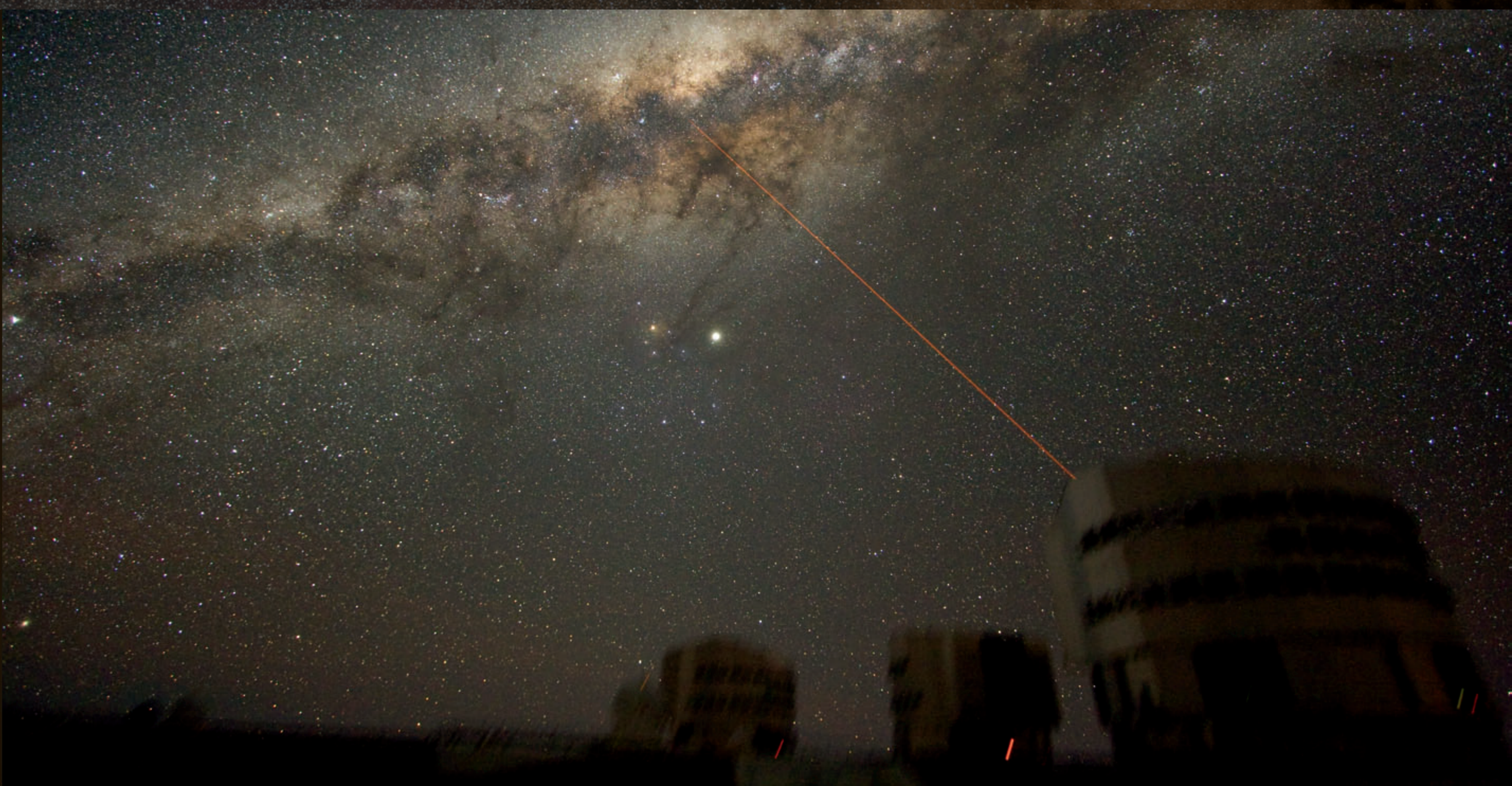
The night sky above Paranal. The VLT is observing the centre of the Milky Way. The laser beam produces an artificial guide star for the VLT's adaptive optics system. Credit: ESO/Y. Beletsky.
