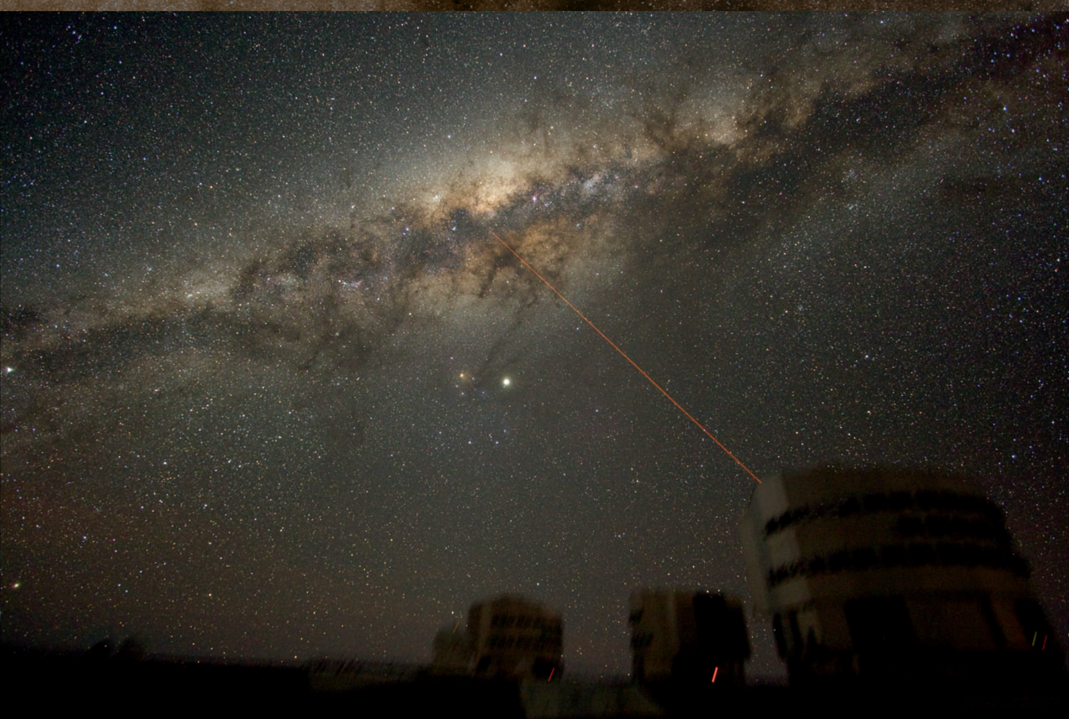
The night sky above Paranal. The VLT is observing the centre of the Milky Way. The laser beam produces an artificial guide star for the VLT's adaptive optics system. Credit: ESO/Y. Beletsky
