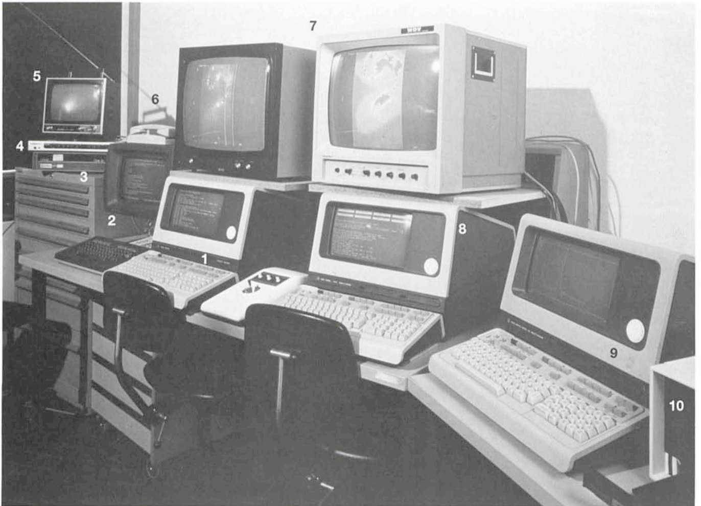
Figure 2: The remote control room for the 2.2-m telescope in Garching. 1 = messages from La Silla, 2 = messages to La Silla, 3 = modem, 4 = TV images receiver, 5 = field acquisition TV monitor, 6 = phone, 7 = Ramtek monitors, 8 = instrument console, 9 = graphic console, 10 = hard copy.
