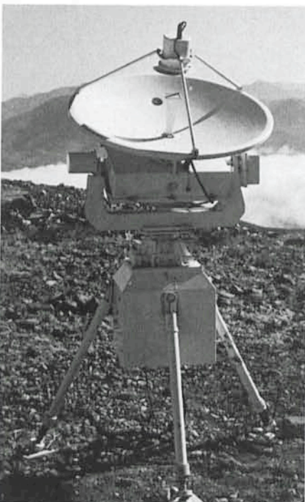
Figure 2: Radiosonde tracking system.
