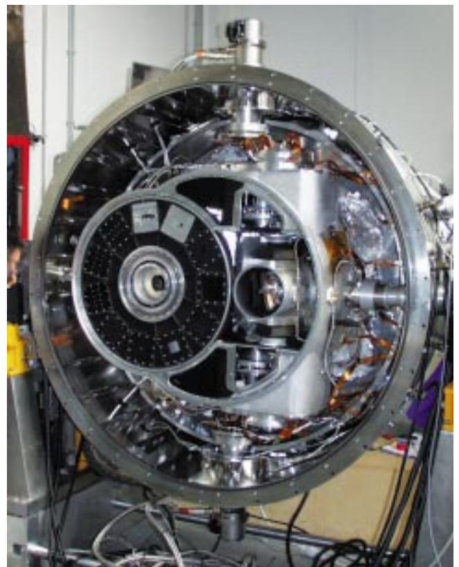
Figure 3: ISAAC with its front vacuum flange removed revealing the slit/mask wheel and the casting used to support its various opto-mechanical functions, including the two cameras which are partly visible to the upper and lower right of the centre.
