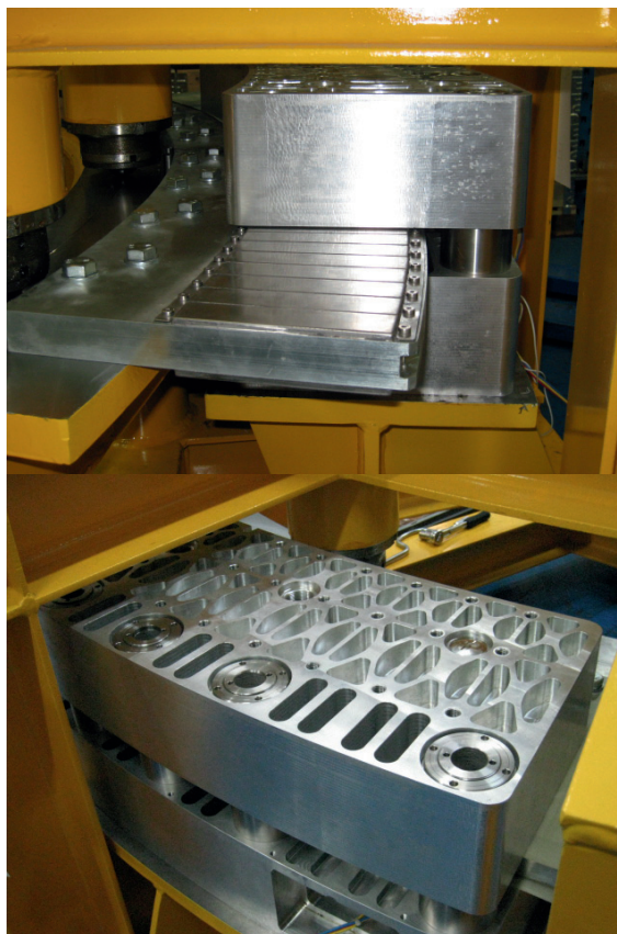
Figure 1: Two views of the linear azimuth motor of the AEM antenna inside the qualification test bench. (Courtesy of EIE/AEM Consortium/Phase Motion Control).
