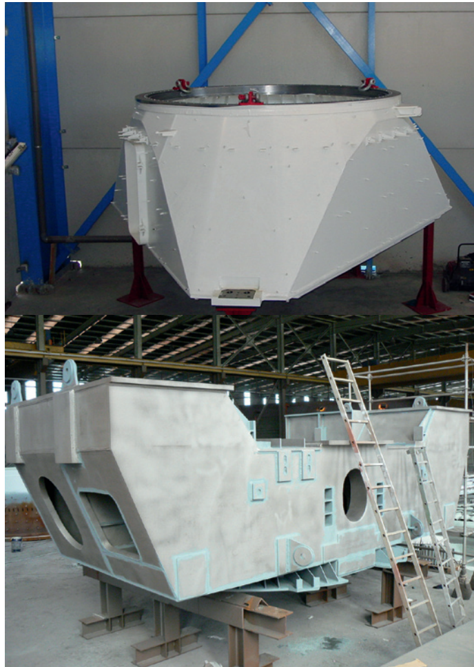
Figure 5: AEM base (upper) and yoke (lower) in manufacturing (Courtesy of AEM Consortium/Asturfeito).
