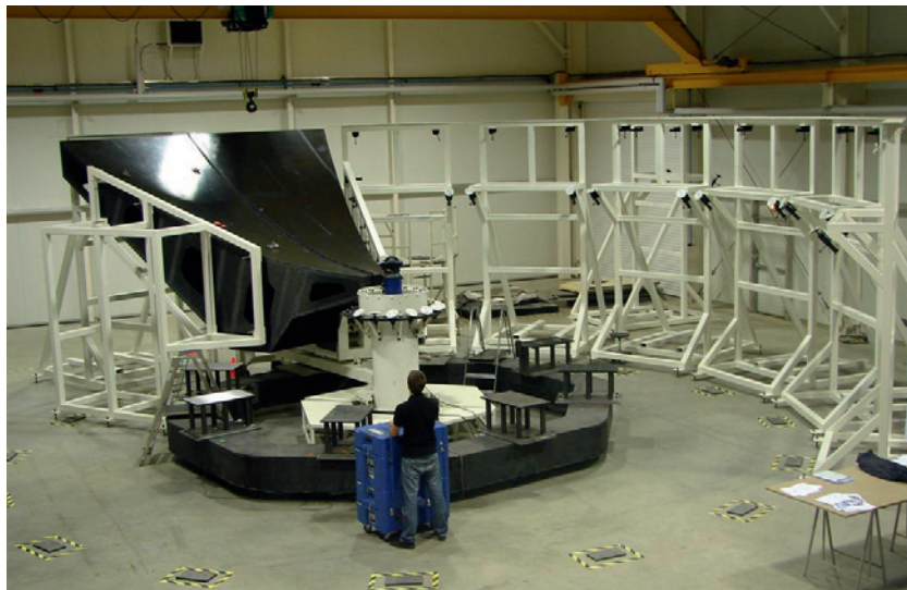
Figure 7: Assembly of the BUS of the first AEM antenna. (Courtesy of AEM Consortium/Duqueine Composites).
