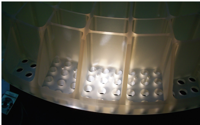
Figure 4. Part of the DSM reference body made by SESO in France (see the image on p. 4, upper, for the whole DSM). The intricate rib structure is literally sculpted from a monolithic block of Zerodur. The 1170 circular holes allow passage for the actuators. This process, known as lightweighting, reduces the mass by 80% to a mere 35 kg.
