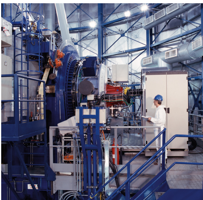
Image of NACO at the Nasmyth focus of VLT UT4 (Yepun). NACO consists of the adaptive optics module NAOS mated with the near-infrared imager and spectrograph CONICA.
