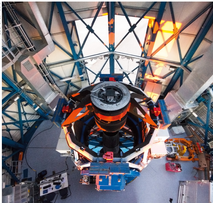
Figure 2. The VST from above. The M1 cover is open and the primary mirror is visible with its baffle. On top, the back side of the hexapod driving M2 is visible. The observation doors with the wind screen are seen on the right side of the picture.
