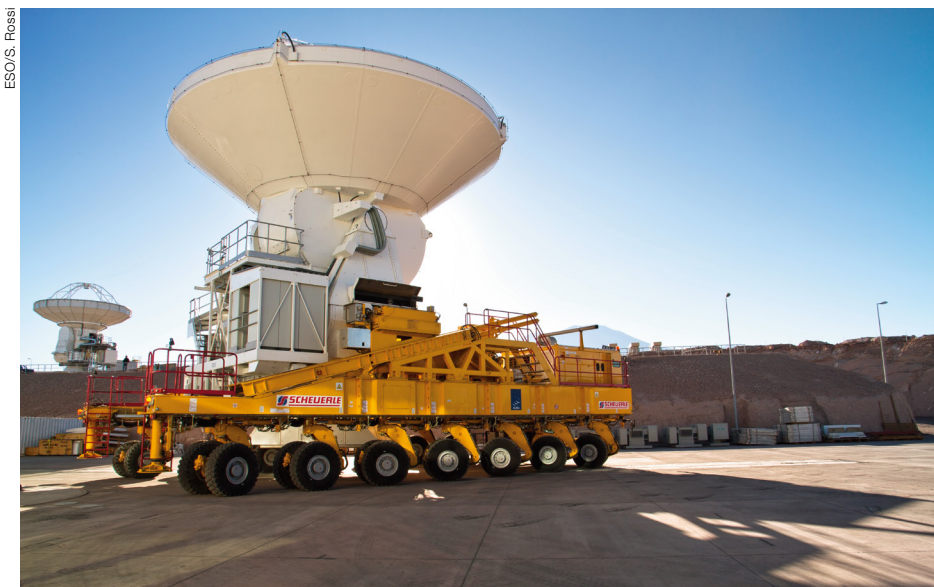
One of the ALMA 12-metre-diameter European antennas is shown being moved on the antenna transporter during testing at the ALMA Operations Support Facility. See Picture of the Week 16 July 2012 for more information.
