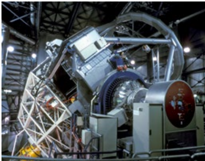
Figure 6. ISAAC at the VLT (UT1). This multimode 1–5 \mu\text{m} imager/spectrometer/polarimeter built by ESO was the first infrared instrument installed on the VLT in 1998 and is still operational and in high user demand. The box attached to the vacuum vessel houses the detector electronics and can be compared with the size of the amplifiers used on the early photometers in Figure 1. The unit in the foreground is the co-rotator needed to avoid tangling the large number of cables and high pressure He hoses for the closed cycle coolers, as the instrument itself rotates at the Nasmyth focus. On its rear is a diagram of the optical layout inside the vacuum vessel.
