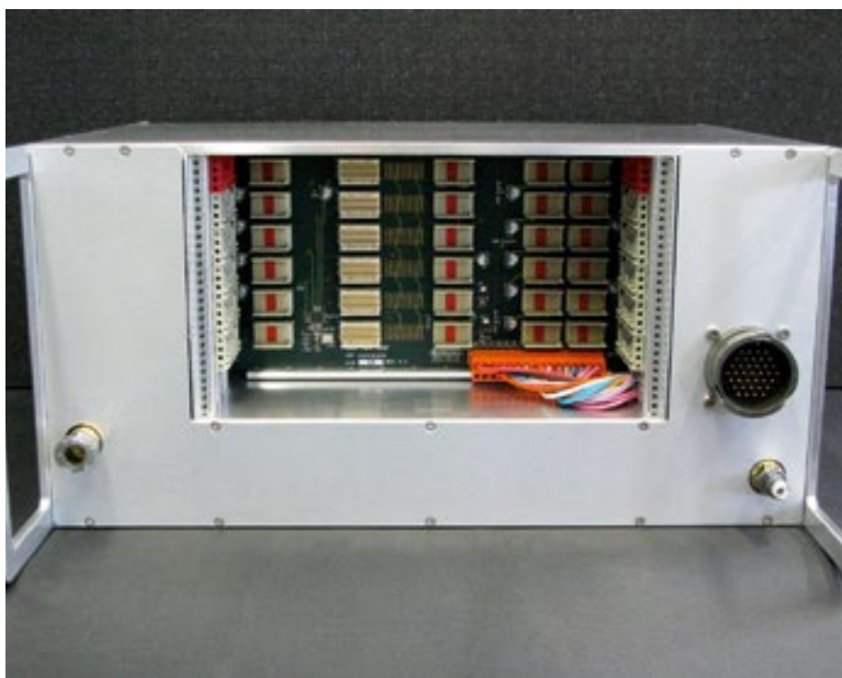
Figure 3. Rear side of an NGC housing with connectors for power cable and cooling-liquid hoses. The width is about 440 mm; depending on application, all surfaces can be anodised. Also visible are the backplane and, on both sides, rails to guide and hold the boards, of which there may be up to six.
