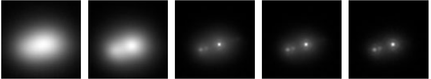
Figure 1. Pictorial representation of the image selection process of Lucky Imaging. The image in Figure 1a is the sum of 50000 z-band images each of 25 ms duration. Figure 1b shows the result of combining the 50000 images, but with shifting to align the centroid of each image. Figures 1c through 1e show the results of selecting the best 50, 10 and 1% of the images according to the Strehl ratio. See text for details.
