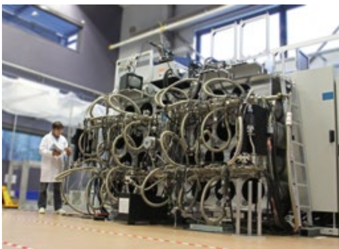
Figure 3. Rear view of MUSE in the CRAL integration hall, showing the large cryogenic system in charge of cooling and vacuum control for the 24 cryostats. The large IFU holes in the main structure are visible between the cooling cables.
