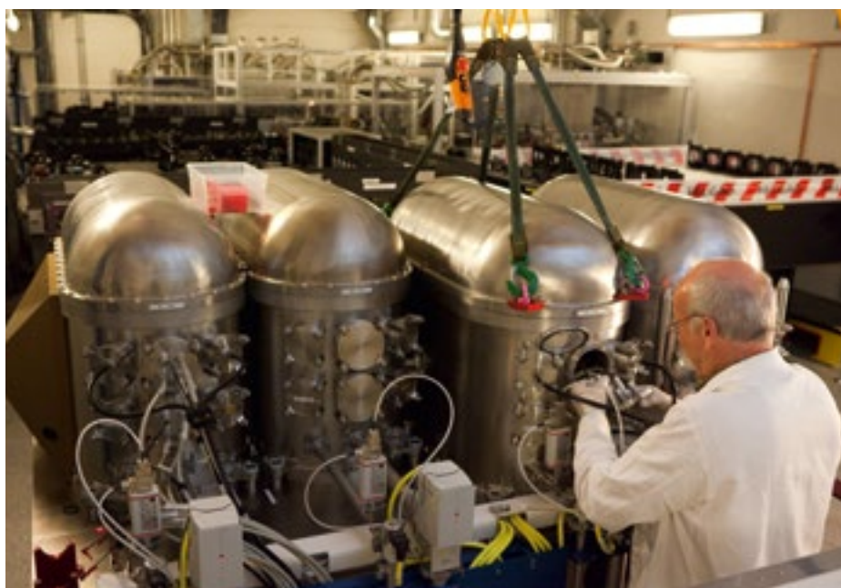
A photograph from 2009 showing the Very Large Telescope Interferometer (VLTI) laboratory at the Paranal Observatory. In the foreground, undergoing maintenance, the differential delay lines of the PRIMA (Phase Referenced Imaging and Microarcsecond Astrometry) instrument are seen.
