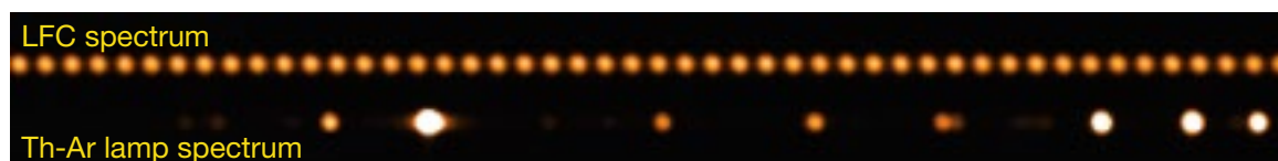
Figure 3. A comparison of a portion of one order of the LFC and the Th-Ar lamp as seen by HARPS.
