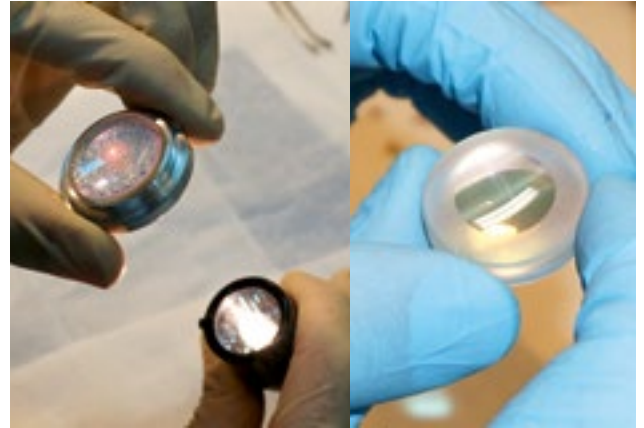
Figure 12. The damaged coating on a SINFONI lens (left) was discovered during inspection after a thermal cycle. The coating was polished away and the lens re-integrated (right).
