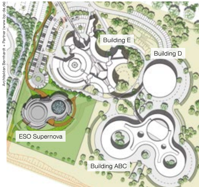
Figure 12. Map of ESO Headquarters in Garching. Building E is the original Headquarters building, connected by bridge to the extension Buildings ABC (containing offices, a larger auditorium, and a new Council Room) and D (the Technical Building, containing a new, larger integration hall).
