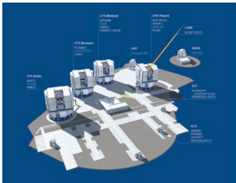
Figure 2. The Paranal system of telescopes and current instruments is shown, with the replacement instruments planned for 2017–2018 indicated (in italics).
