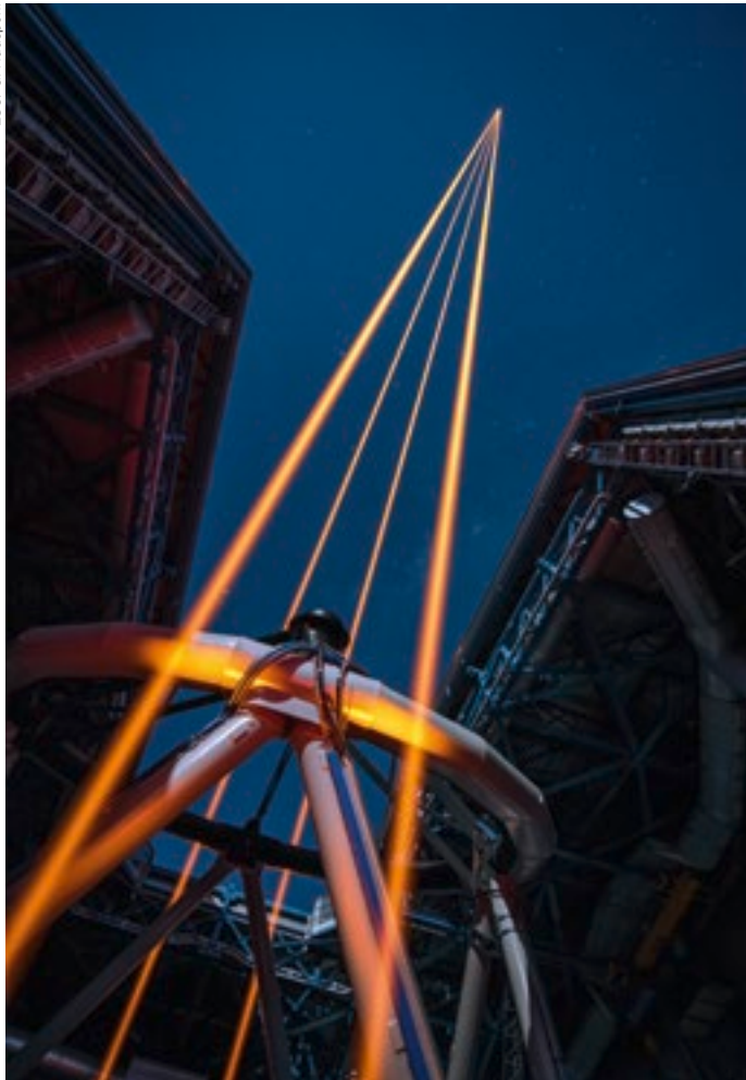
Figure 5. The four laser guide stars of the Adaptive Optics Facility on VLT Unit Telescope 4.
