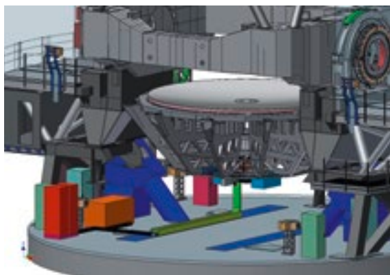
Figure 2. (Left) Cables and He lines routed from the M1 cell through a chain (green) to electronics cabinets (red) and helium compressors (orange). This configuration is very similar to the baseline design accepted at the VISIR Final Design Review in 1999.
