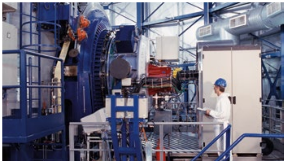
Figure 1. NAOS (light blue) and CONICA (red) are attached to the Nasmyth B adapter of UT4 (Yepun). The control electronics are housed in the white cabinets.
