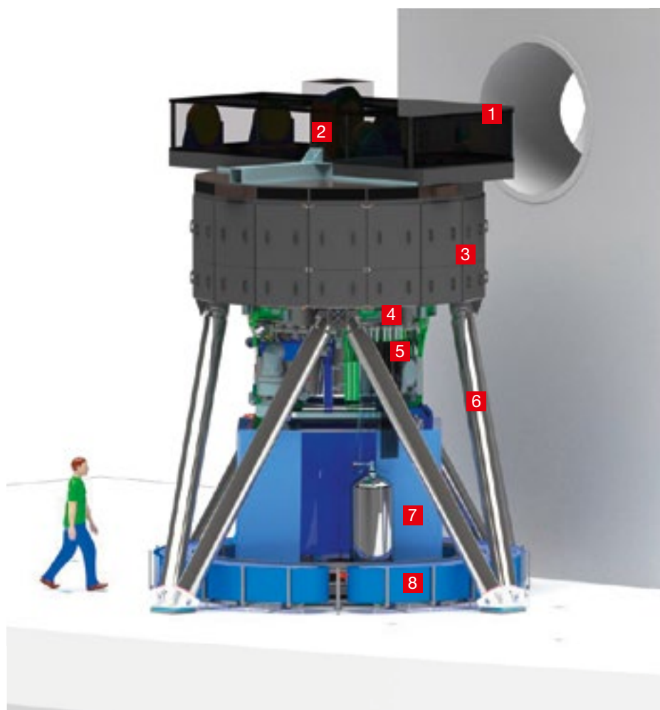
Figure 3. Rendering of MICADO in a stand-alone phase before it is integrated next to MAORY. The pre-focal station, which transfers the optical axis horizontally at a height of 6 m above the Nasmyth Platform, is indicated by the grey block. The key components of MICADO are labelled, and a person is shown for scale. For a view of MICADO in its final location next to MAORY, see the accompanying article on the MAORY system (Cillegi et al., p. 13).
