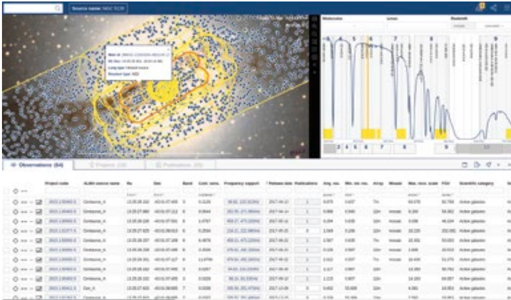
Figure 4. The ASA query interface features search-as-you-type, a sky view, a spectral coverage viewer, a result table, and much more. All objects from SIMBAD and NED falling into any of the regions of the ALMA observations are displayed and even the object-types can be queried for.
