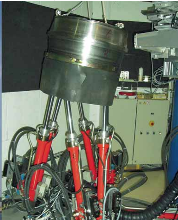
... and the 120kg central roller bearing being measured using neutron diffraction
