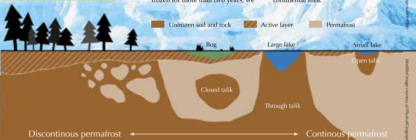
Figure 2: Cross-section showing different types of permafrost
