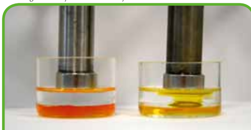
Figure 4: The effects of a magnet on solutions of normal (left, with added dye to show the two layers) and magnetic (right) surfactants. The presence of iron in the magnetic surfactant explains the attraction seen on the right.
