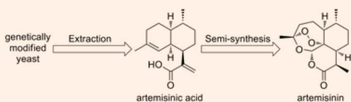
Figure 4: The extraction and semi-synthetic synthesis of artemisinin from genetically modified yeast
