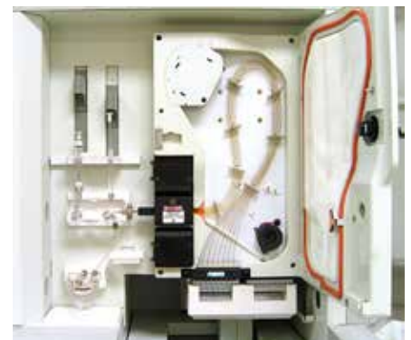
A DNA sequencer, showing the capillary array and blocks and syringes.
