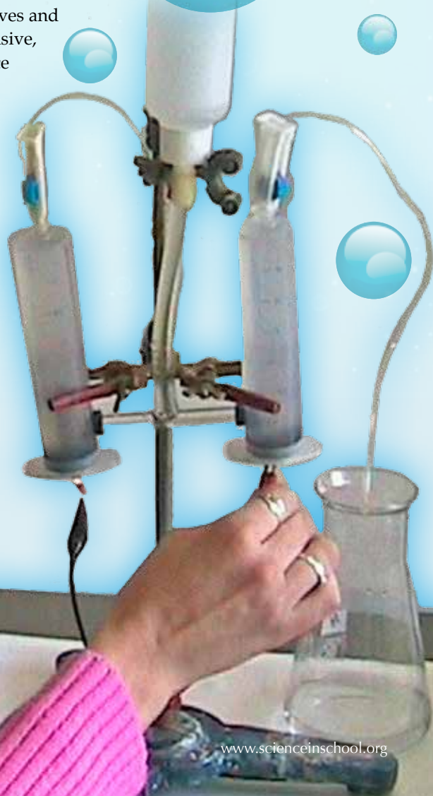
Figure 1: Connection of the electrolyser electrodes to a solar panel
