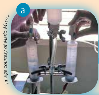
Figure 4: a) Opening the valves to allow the gases to pass to the electrodes of the fuel cell; b) electricity generation by the fuel cell
