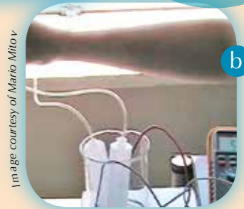
Figure 4: a) Opening the valves to allow the gases to pass to the electrodes of the fuel cell; b) electricity generation by the fuel cell
