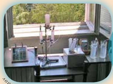
Figure 7: Prototypes of water electrolyser, fuel cell and gas holders
