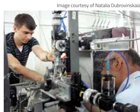
Image courtesy of Natalia Dubrovinskaia Maxim Bykov and Leonid Dubrovinsky preparing a diamond anvil cell experiment with laser heating at ESRF
