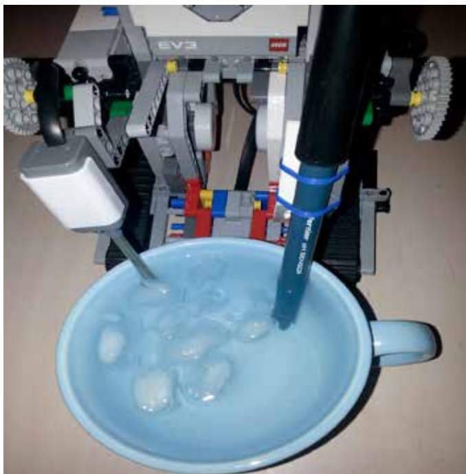
Chembot embedding its sensors into cold water to take measurements of temperature and pH
