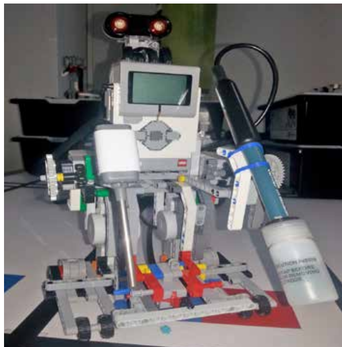
A finished Chembot, complete with sensors
