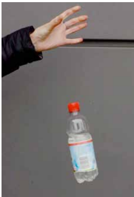
Figure 2: letting the bottle fall: water stops flowing out.
