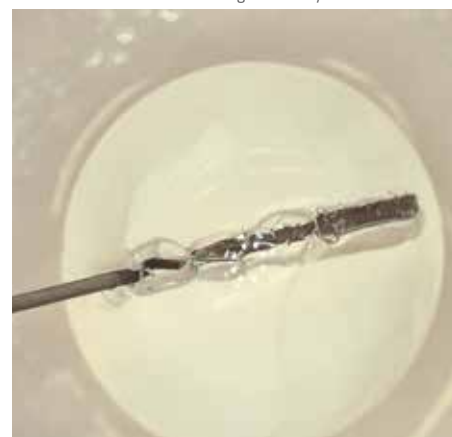
Figure 5: hydrogen gas bubbles appearing during the electrolysis of water
