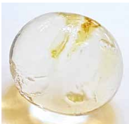
Figure 3: reactions in hydrogel balls: (i) iron(III) chloride with sodium hydroxide
