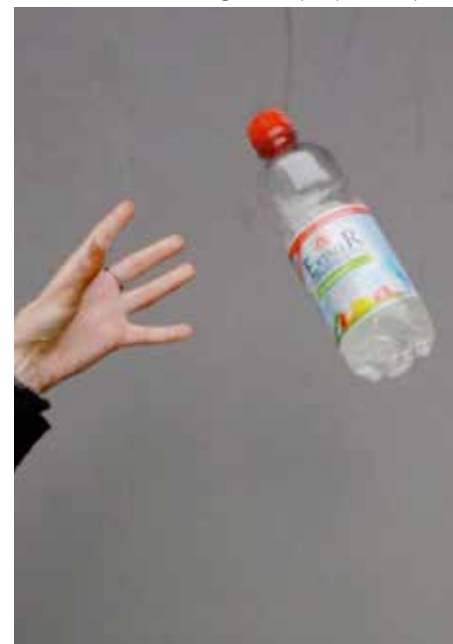
Figure 3: throwing the bottle upwards and letting it fall down: no water flows out during the upwards or downwards motion of the pierced bottle.
