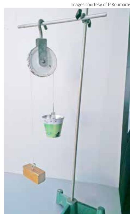
Figure 4: the experimental set-up with block, bucket and pulley
