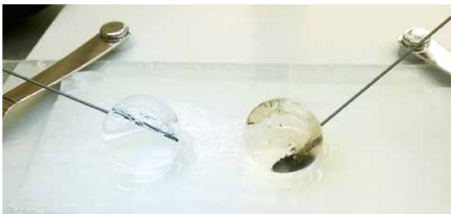
Figure 4: electrolysis of silver nitrate solution in a hydrogel ball
