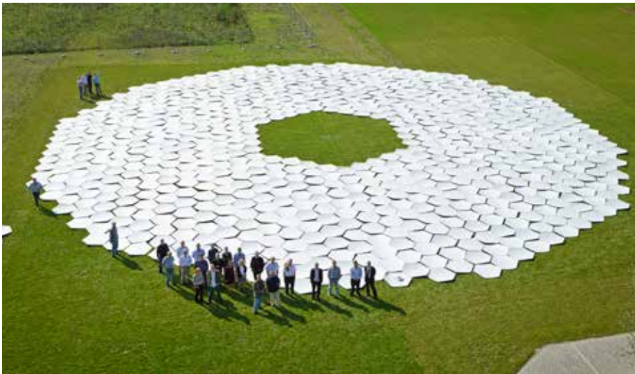
A scale mock-up of the ELT primary mirror, using cardboard versions of the mirror segments
