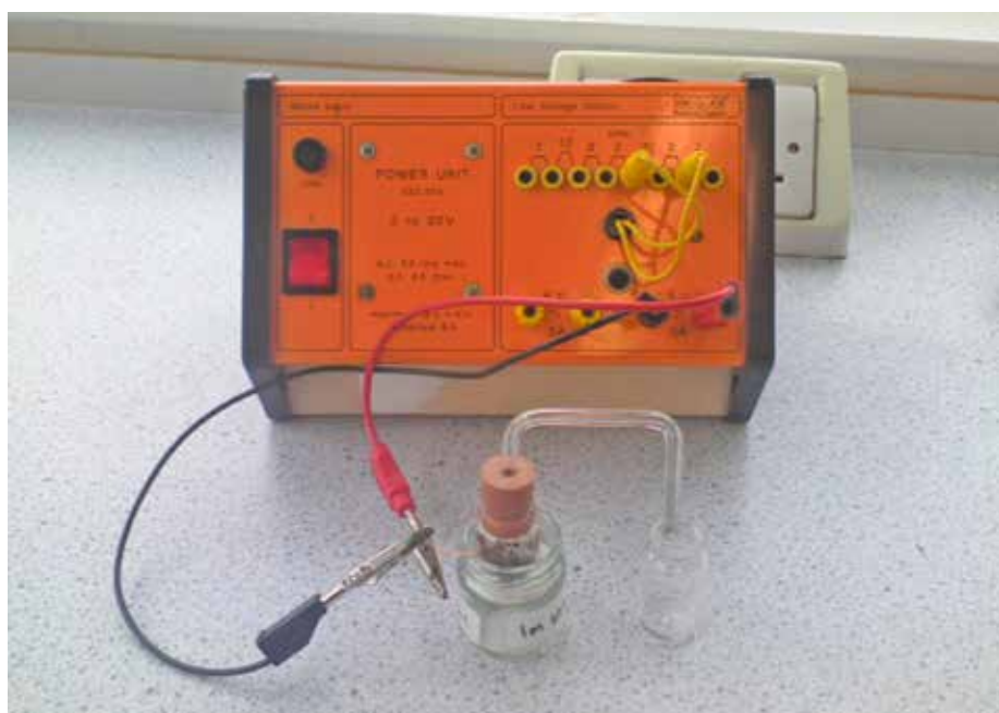
Figure 4: Experimental setup showing the microscale heater connected to the power supply
