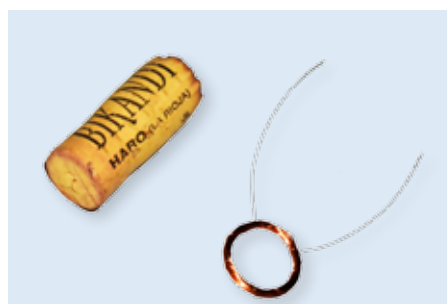
Figure 2: The coil for the loudspeaker is created by winding copper wire around a wine cork.
