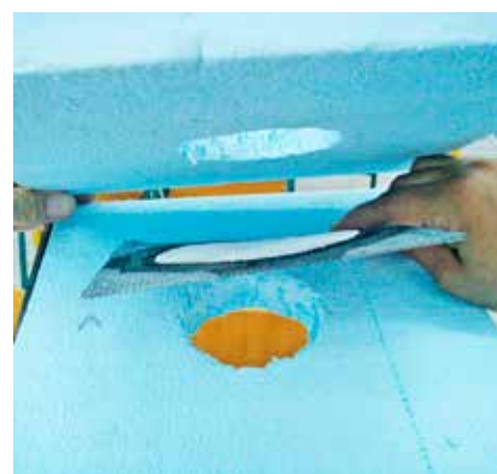
Figure 4: The wire gauze mat is sandwiched between the two thinner polystyrene pieces.
