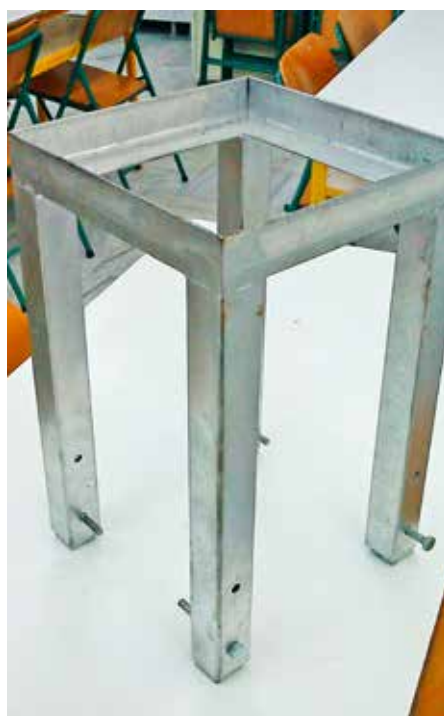
Figure 2: A metal base, such as this, acts as the main support for the calorimeter.
