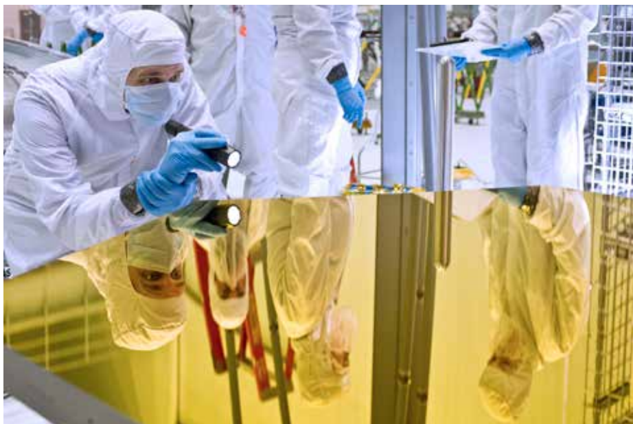
Inspecting the hexagons of beryllium that will make up the primary mirror of the James Webb Space Telescope
