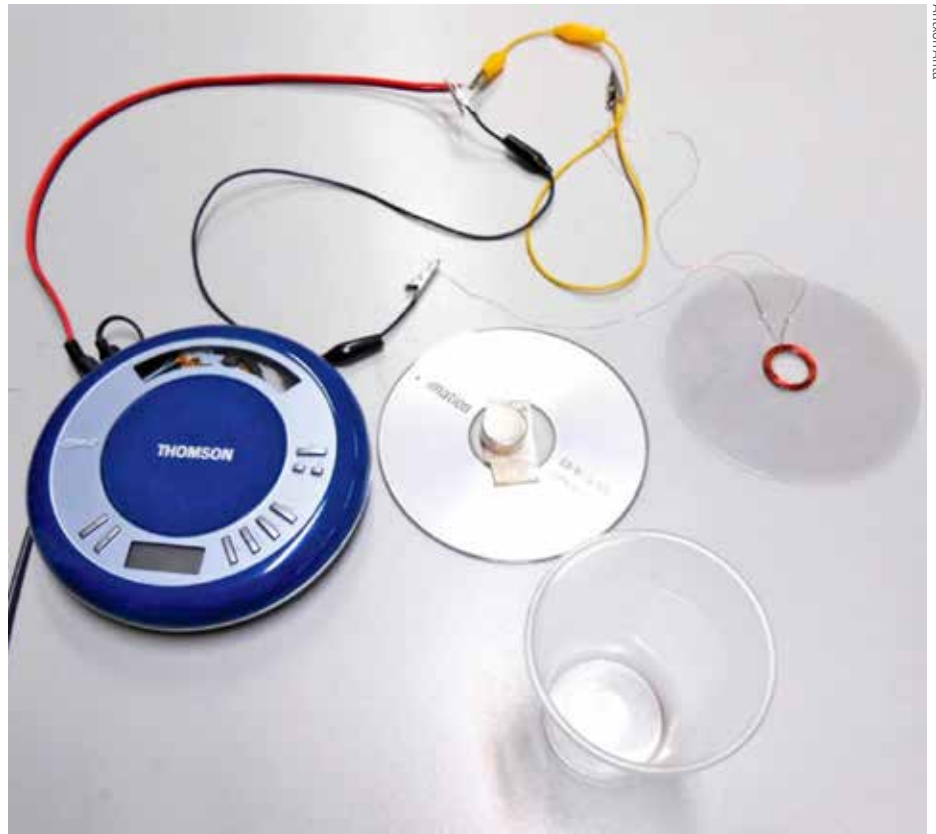
Figure 5: The components of the loudspeaker, using an mp3 player for the audio source
