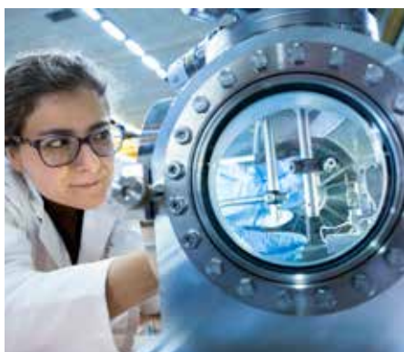
A scientist adjusts a fine liquid jet containing samples of viruses, cells or bacteria inside a vacuum chamber, so that they can be probed by X-ray laser flashes at European XFEL.
