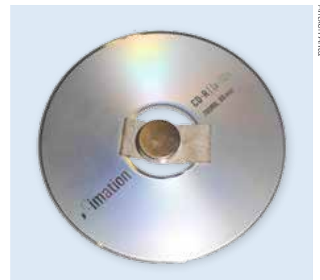
Figure 4: Using tape or glue, the magnet is fixed to a CD for support.
